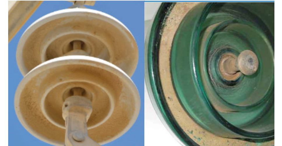
C&P insulators with pollution accumulation on underribs
